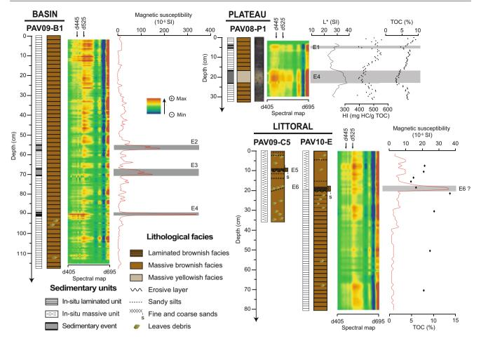
**Fig. 22.8** Multidisciplinary characterization of Lake Pavin sediments retrieved by short gravity cores, in the deep central basin (PAV09-B1), on the plateau (PAV8-P1) and in littoral environments (PAV09-C5 and PAV10-E). Visual descriptions of sedimentary facies are further defined (i) by sediment diffuse spectral reflectance (here plotted on a 3D diagram where the X axis represent the wavelengths, Y is the depth in core and Z the first derivative value for the corresponding wavelength (in
