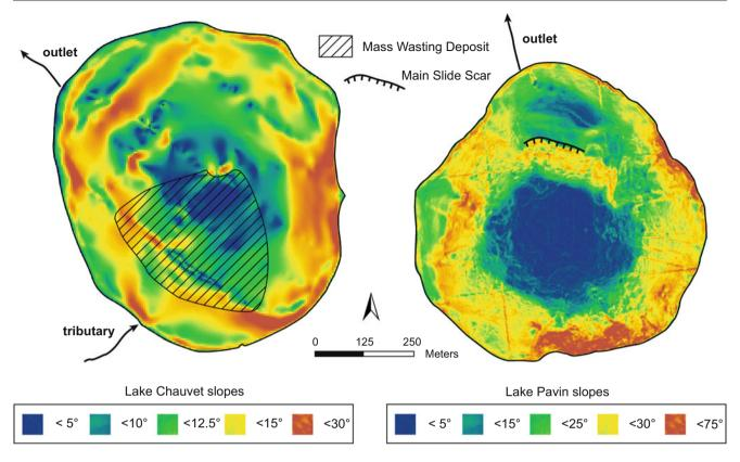
Fig. 22.7 Slope maps of maar lakes Chauvet (left) and Pavin (right)
